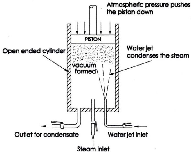
Steam enters the cylinder and its pressure pushes the piston to the end of the cylinder. The jet-stream of water condenses the steam, which lowers the steam pressure because the steam is now colder. The piston therefore retreats again to the front of the cylinder.
